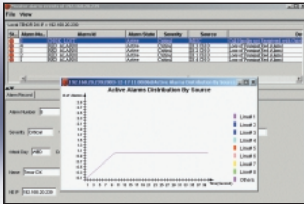
Tenor Monitor Alarm Events screen shot. Chart depicts Status, Alarm Number, ID, State, Severity, Source and Description.
